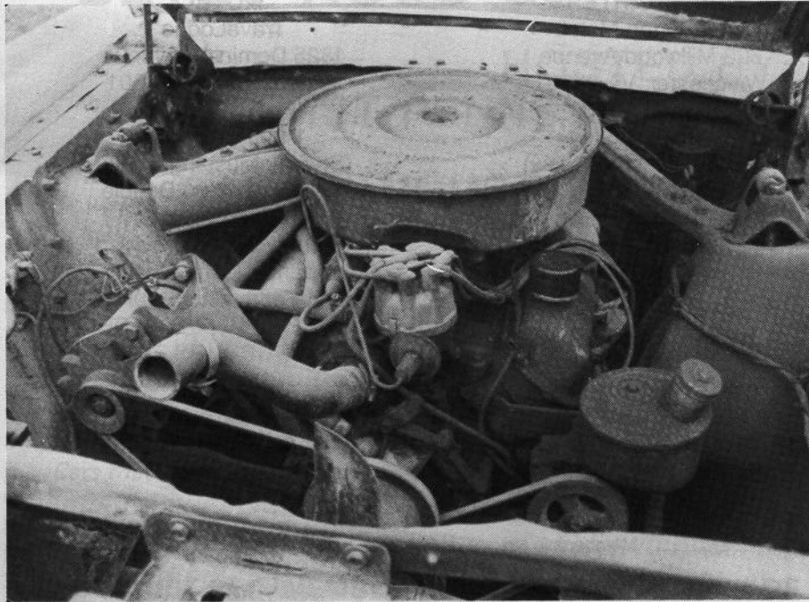
Most Pace Car engine compartments need some detailing but some are otherwise perfect. Note the correct Eaton power steering, generator, and oil filler cap on the valve cover.
