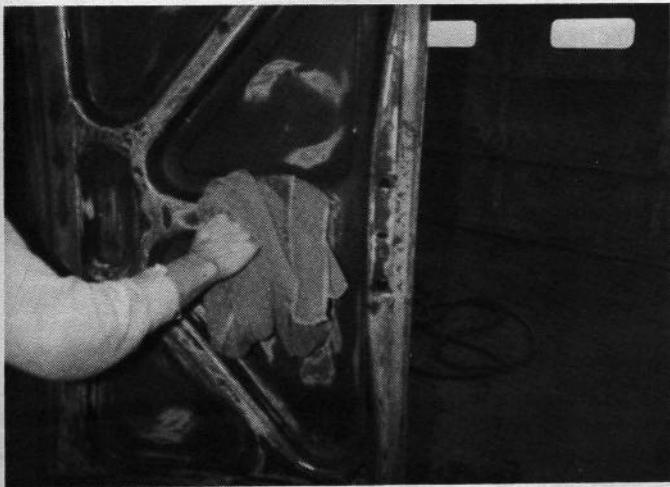
The metal surfaces are wiped dry with a clean absorbant towel.
