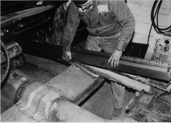
Skinner positions the inner rocker box for permanent installation. When it comes to structural integrity, this is probably the most important component of all. Measurements must be taken and door fit must be perfect.
