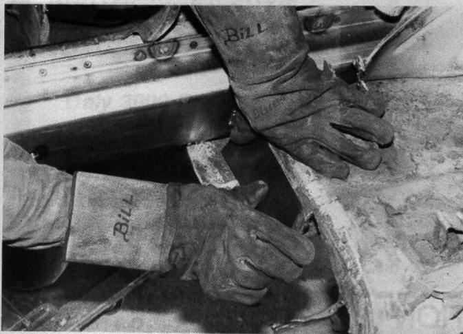
Next, Skinner takes a piece of stock and checks for fit. This piece will have to be formed into place using a penning technique.
