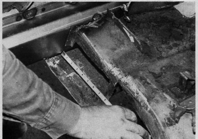
With our inner rocker box welded in place, we're ready for other areas. Skinner measures eight-inches for the plate he will fabricate here.
