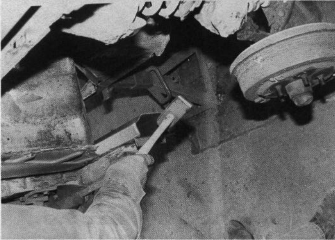
Once in position, the inner rocker box can be adjusted with the gentle tap of a hammer. Sometimes it takes a firm blow.
