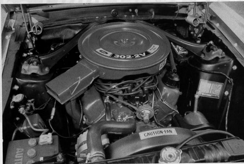
Engine choices for 1970 ranged from the 200 cid in-line six-cylinder to the awesome 429 found in the Boss 429. The F-code 302 2V, as shown here, was rated at a substantial 220 horsepower.
