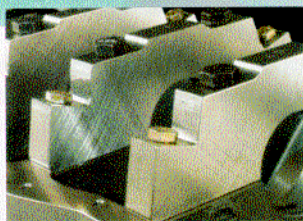
4 bolt main caps on the center three mains
