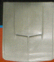
1967-68 Fiberglass Hood with Steel Back
