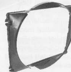
1967-70 Mustang radiator shrouds made from original Ford tooling
