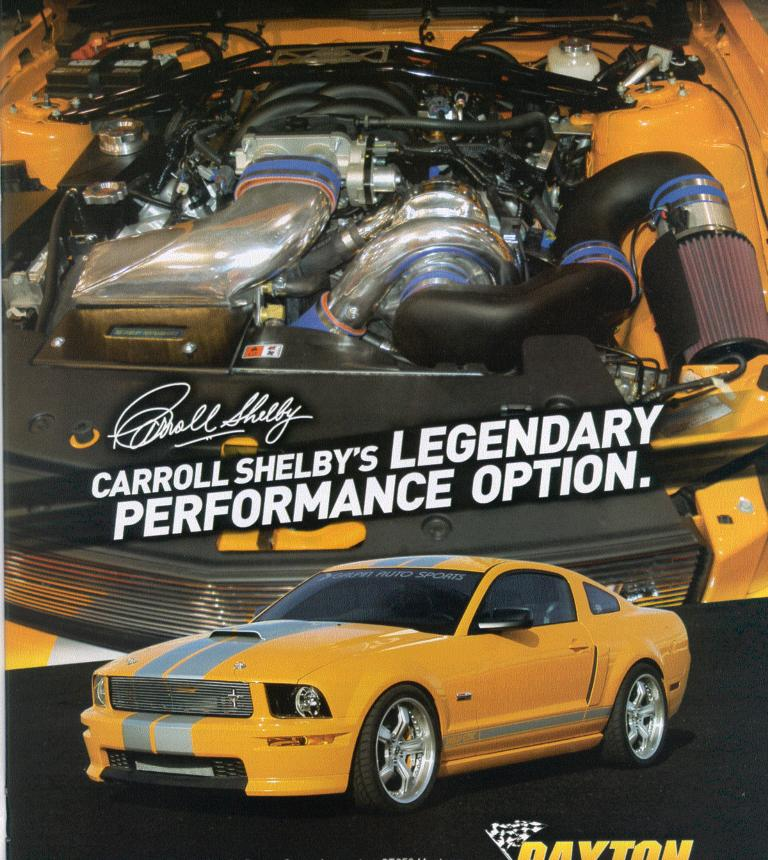
In 1966, Carroll Shelby fitted a Paxton Supercharger to a GT350 Mustang and the rest was history. Experience the same thrills and chills as Shelby himself with this modern-day air/water charge cooled Paxton NOVI-1200 centrifugal supercharger system. 2007-08 Mustang Shelby GT/SC 462 HP.
