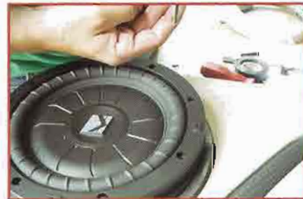
▲ Screw the speaker to the spacer, install insulator and bolt on the back.
