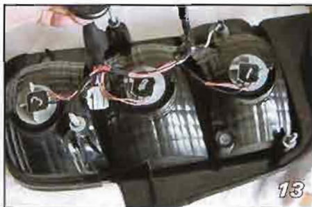
▲ As mentioned, the harness is clearly marked. Number 1 is the inner light, 2 is the middle, and 3 is the outer.
