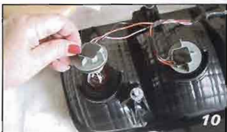
▲ Remove the sockets from the taillight housing by twisting each to detach them from the housing.
