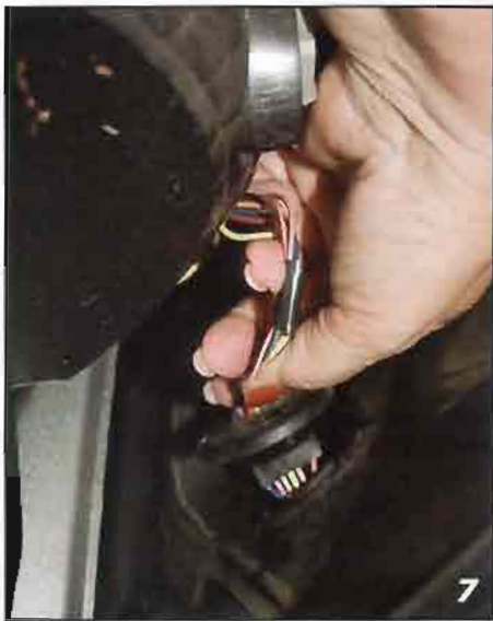
▲ Remove the taillight housing from the Mustang.
