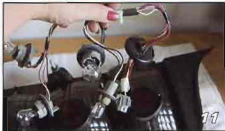
▲ Remove bulbs from the factory harness for reuse with the sequential harness. If you touch the bulbs with bare hands, wipe each bulb with isopropyl alcohol to remove oil your hands and fingers to prevent bulb burnout.
