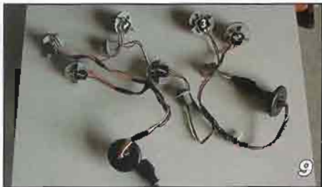
▲ The assemblies are interchangeable. Harness socket are labeled, 1, 2, and 3.
