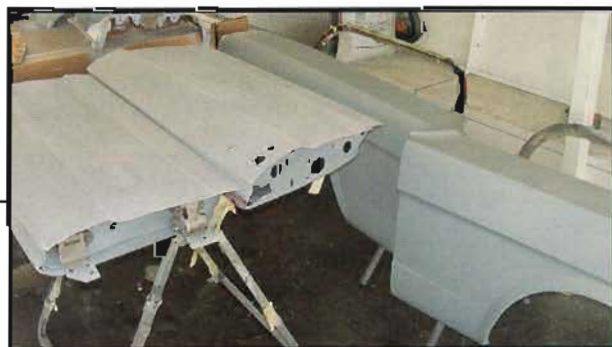
These parts are primed and ready for final sanding before applying paint. The paint will be the new water-bourne line from PPG, which is ecologically friendly.
