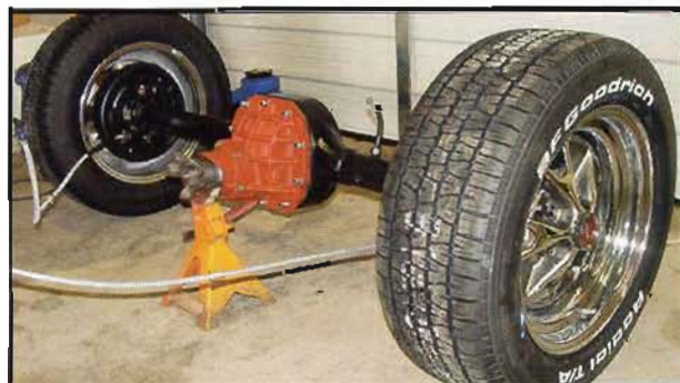
The rear assembly is completed, detailed, and ready for installation. Its new third member and axles are compliments of Currie Enterprises; new rear brakes, Styled Steel Wheels from Scott Drake Automotive Group; and new BF Goodrich Tires are compliments of Bill Day Tire Company, Tyler, Texas.
