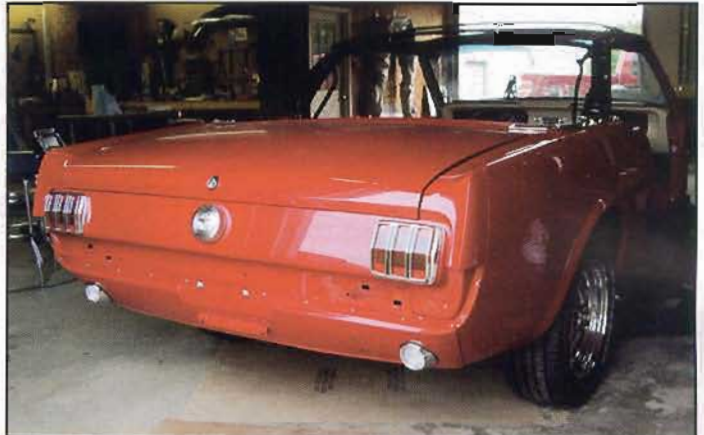
This photo shows the back of the car after the rear suspension, deck lid, rear valance, and back up lights are installed.
