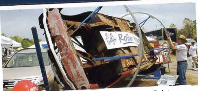
DSK Auto Products and Auto Kraft Body & Paint owner Doug Kilien developed this Roller Hoop body rotation system. Look for more on this in an upcoming issue.
