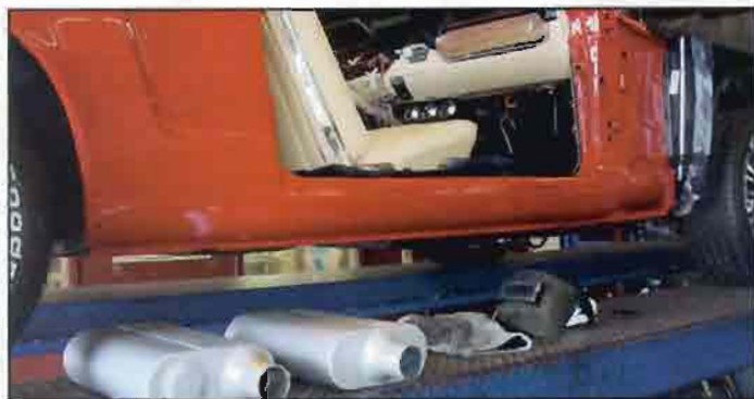
The car is placed on a lift for installation of a Flowmaster Delta 40 series dual exhaust system. After installation, it sounded really great.
