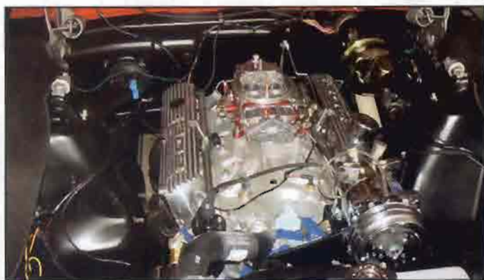
The engine is placed in the car and ready for accessories and brackets. It is a 302 roller motor with Ford Racing aluminum heads and intake provided by Quantum Performance and a performance carburetor provided by Ortigo Performance. The polished air compressor is part of the package donated by Old Air Products.
