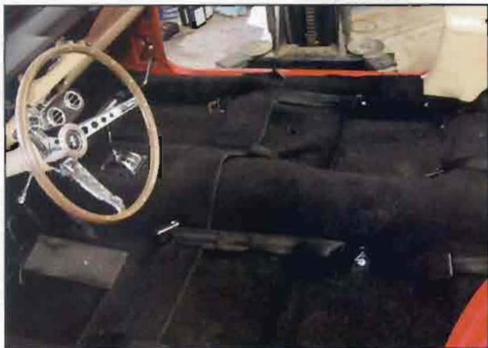
The underlayment, carpet, and seat belts are installed in preparation for the seats, kick panels, door panels, etc.
