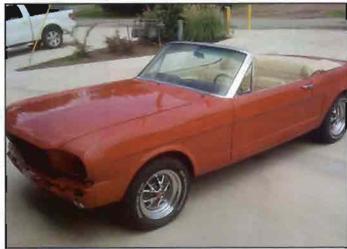
The hood, doors, fenders, and front end are assembled on the car. It is now ready for the front bumper, headlights, grille, and fog lights.
