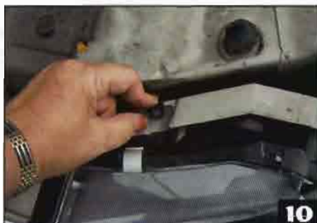
▲ Next the first of two headlight retaining clubs in pushed back into place.
