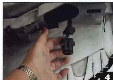
▲ After the assembly was released from the Mustang, the headlight bulb connector was removed from the headlight.
