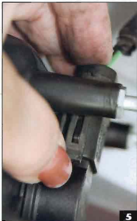
▲ Next, the clip on the electrical connector on the sidemarker bulb was released.
