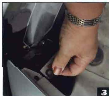
▲ First, the retaining clips, long slender clips that hold the headlight to the panel, were removed.
