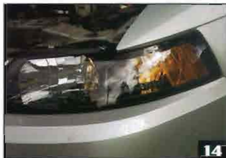
▲ Both headlights are replaced. It's a good idea to get them aligned properly. We connect the battery and tested the lights.
