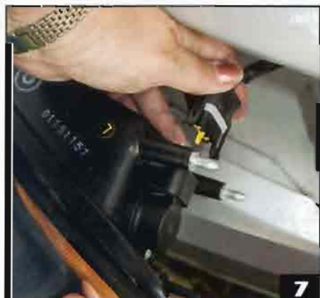
▲ The sidemarker connector was first reattached by simply pushing it until the clip snapped into place.
