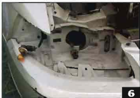
▲ Once the headlight was totally removed from the Mustang, we took the opportunity to give the area a good cleaning.
