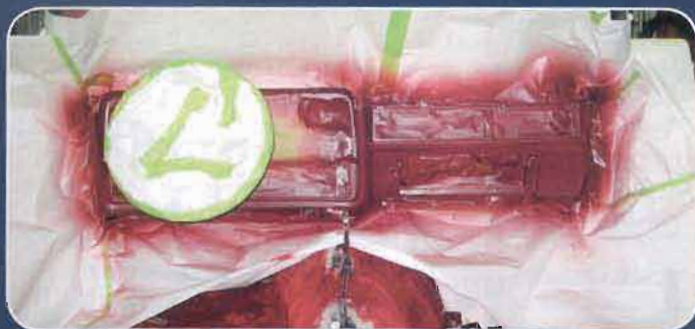
▲ To make sure everything inside the car matched properly, R&A refinished the dash panel in the same dark red as the various interior panels.
