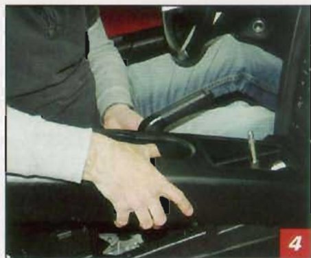
▲ Tilt the console forward to clear the emergency brake, remove the console.
