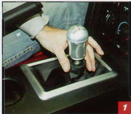
▲ Place transmission in neutral, engage the emergency brake fully. Push the boot down and remove the shift knob.
