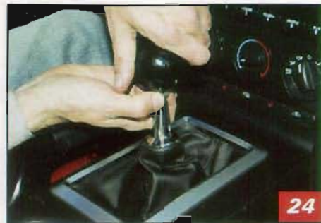
▲ A new shift ball bearing an MGW logo was screwed into place and the lock nut was tightened.
