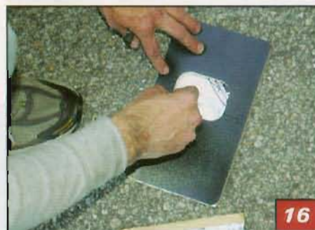
▲ Using the supplied insulation blanket as our template, Dustin trimmed the supplied Dynamat insulation to fit.
