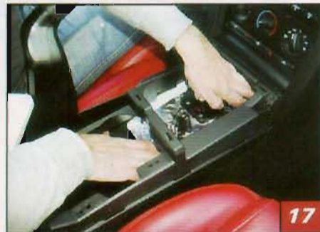
▲ Peel the backing away and press the Dynamat into position.
