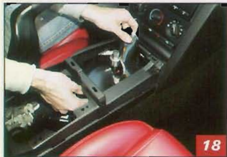
▲ Place the foam insulation into position. There are two slits on the rear of the insulation that slip over two bolts to properly align it and hold it in place.
