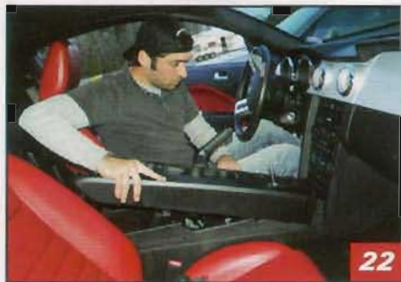
▲ Dustin gently replaced the center console and tightened it up with the two screws.
