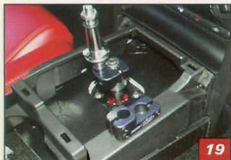
▲ Two shift handle brackets are included in the kit. Bill chose the shorter one as his position felt most natural to him.
