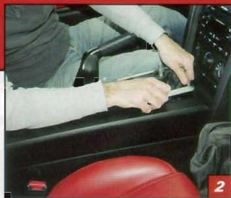
▲ Gently remove the shifter boot and trim ring. It just pops up. Don't be afraid, it won't break.
