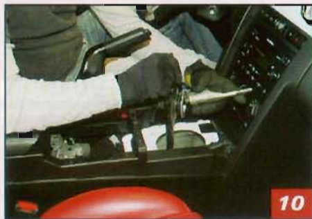
▲ Back inside the car, remove the shifter. Push the shifter as far forward as possible, then lift the rear of the shifter through the opening.
