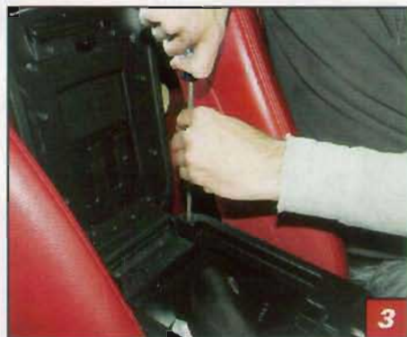
▲ Two screws hold the entire center console in place.
