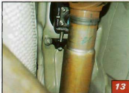
▲ Slip the MGW Shifter into the rear support, then tighten the bolts on the rear support.
