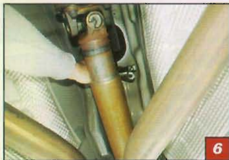
▲ Now it's time to go under the car. A good trouble light will make it easier to see all of the parts, as the transmission and exhaust pipes are in the way. Remove the rear support bracket.
