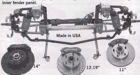
There is no need for tower supports. The rear steer crossmember that holds the rack sits above the bottom of the oil pan.
