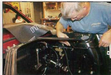
▲ Marty works on the wiring harness installation.
