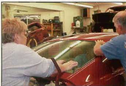
▲ With Jeff working inside, Marty and I pressed down on the rear window as it was installed on the Mystical Build.
