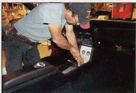
▲ Jeff installs the center console made and donated by Peter Faull of Canada.
