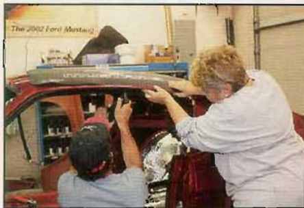
▲ Jeff bolts in trim pieces around the window opening as I held them in place.
