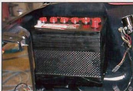
▲ A borrowed Autolite battery, vintage in looks but a gel cell battery inside.
