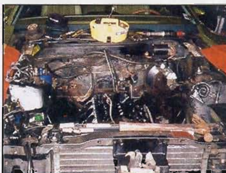
▲ Earl removed the intake and heads to make engine easier to remove.
