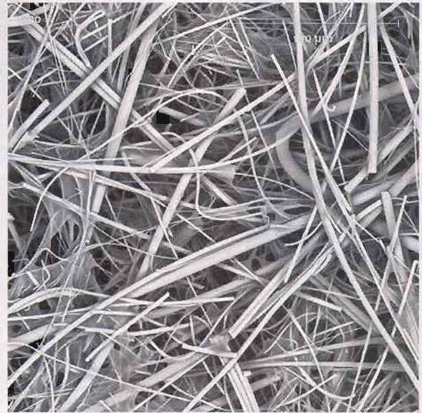
100% Synthetic Glass Filter Media - 1000X Zoom
