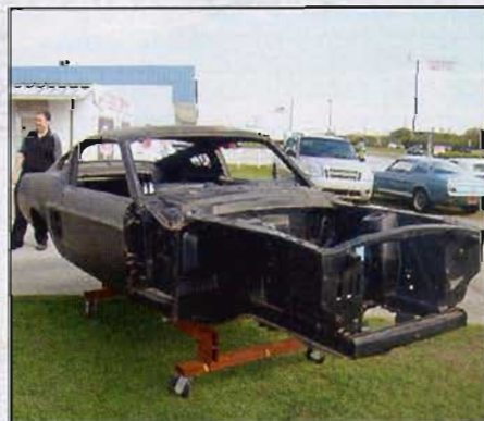
▲ Done! The body now sat on the "dolly" in the proper position, ready to be loaded into the trailer.
