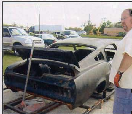
▲ The floor jack came in handy in getting the heavy body off the base onto the "dolly."
