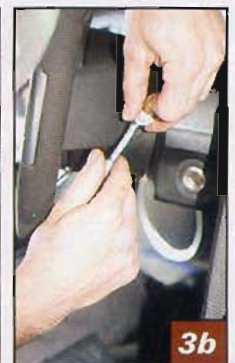
▲ James removed the plastic bolt caps from the sides of the steering wheel by prying them out with a small screw driver. Then he removed the airbag module bolts found underneath these caps with either an 8 or 10mm socket.
