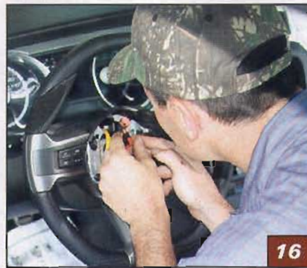
▲ Next, the horn switch assembly was reattached followed by tightening the three T-30 Torx screws securely.
