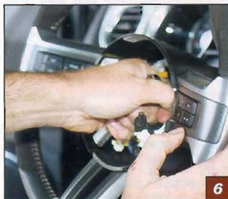
▲ Disconnect the horn by pulling off horn switch at the upper right tab. Disconnect the wheel switch wiring harness at the clockspring column connector.
