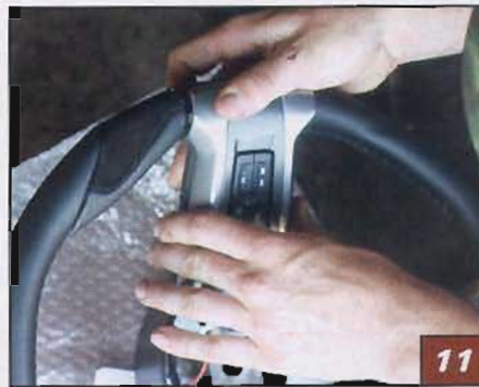
▲ James then installed the three silver spoke trim panels onto the Grant wheel by positioning them above their alignment holes and pushing them down into position. He made sure each panel was securely in place.
