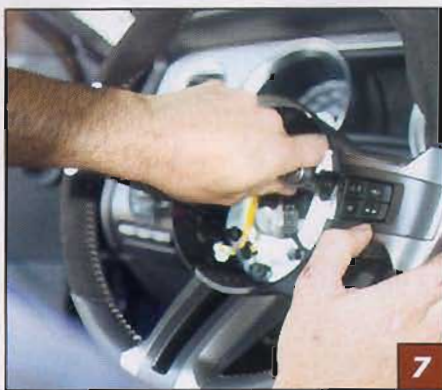
▲ Remove the horn switch after loosening the 3 T-30 Torx screws. Remove the assembly from the wheel. The cruise control switch wiring harness is now exposed and can be removed by using a T-20 Torx driver (screw has a green ground wire).
