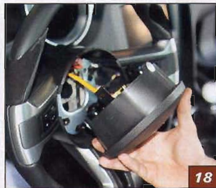
▲ James repositioned the airbag module and reconnected the wire leads.
