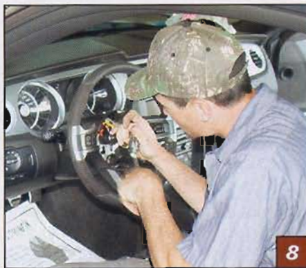
▲ Next, James loosened the steering wheel retainer bolt with several turns, and removed the steering wheel from the column.
