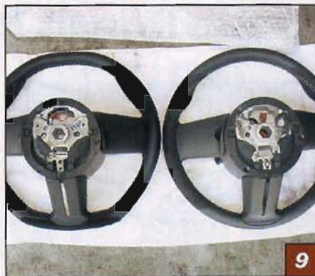
▲ Since the rear plastic shroud on the original and new wheel are identical, James chose not to change the shrouds.
