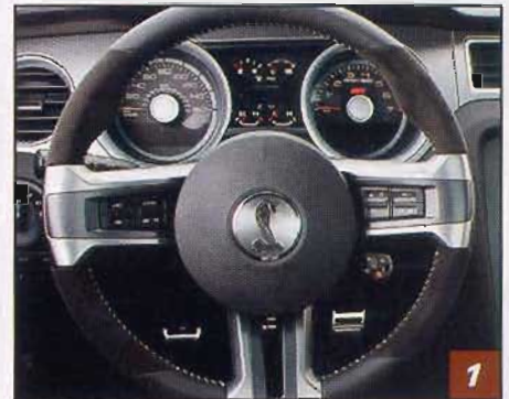
▲ Position the steering wheel so it’s pointed straight ahead. You might want to jot down your radio presets; you will lose them when you proceed with step 2.
