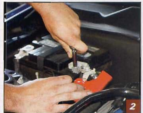
▲ Disconnect the battery. Wait a full minute for the circuit to completely discharge before proceeding.
