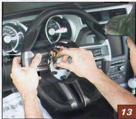
▲ James positioned the new wheel onto the shaft, routing all wires through the opening.
