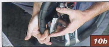
▲ Remove the three silver spoke trim panels. Place your fingers under the trim at the outside end where it meets the wheel, gently pull upward. Once it starts to move, pull it straight up.
