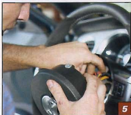
▲ Next, he disconnected the electrical connectors from the airbag module and removed the airbag module from the steering wheel. James placed the module face up on the floor. (Note: If you carry the module, make sure the trim cover is pointed AWAY from your body).
