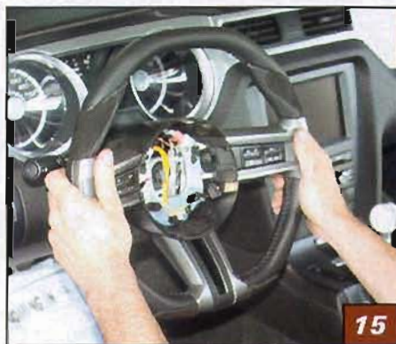
▲ James double checked the wiring harness and installed the green ground lead using the screw which he previously removed, then he tightened it securely.
