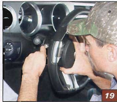
▲ He then positioned the airbag module into the wheel and reinstalled the two airbag module retaining bolts. Again, directions indicate these should be tightened to 62 lb-ft (7 N-m).
