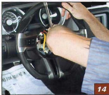
▲ Next, he installed the steering wheel retainer bolt. Directions recommend that it be torqued securely to 41 lb-ft (55N-m).
