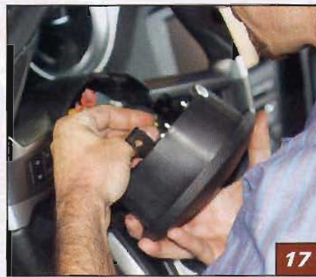
▲ The horn lead was reconnected to the tab on the upper right of the switch. The cruise wiring harness was reconnected to the clockspring mechanism coming from the column.
